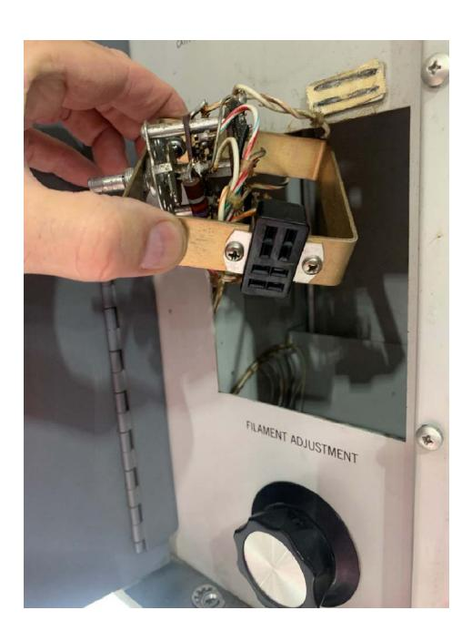
The HV started shutting down, I figured out that the lightning protection circuit was the culprit and found that the capacitor that connects to the tank circuit was intermittently shorting. I disconnected one leg of the cap to continue testing.
