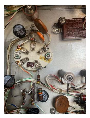
January 10<sup>th</sup>, 2023 AC0MO and I wound a new plate choke on a Delrin core, it measured at 297uh, the original plate choke measured at 2mh and was known to be self-resonant in the 75m band.
