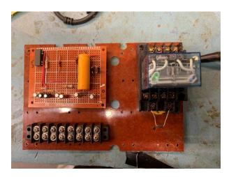
February 4<sup>th</sup>, 2023 I completed and installed the PTT circuit with a sequencer, power supply, and contactor relay.
