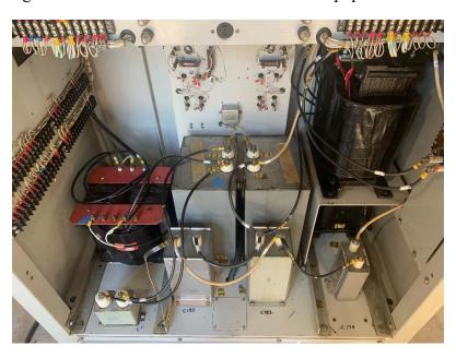
January 15<sup>th</sup>, 2023 When I tried tweaking the oscillator and driver circuits I discovered a problem, no metering, I pulled the metering switch out and found a Jones connector that matched the connector on the mystery cable. Viola, now metering was working along with many other things...
