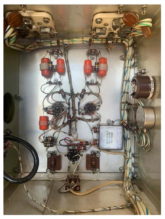
I also added an additional screen bypass for the 807 driver in the RF Deck to eliminate a possible 60Mhz parasitic.
