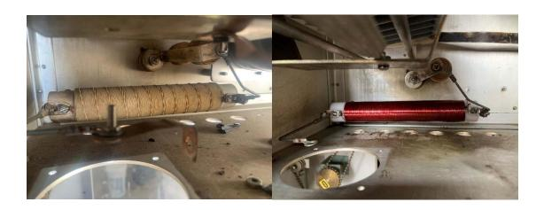
January 11<sup>th</sup>, 2023 We installed the new plate choke into the Tank deck. We also installed new components for the Plate Bypass and RF Feed. I also modified the mechanical passthrough for the plate connections and made the modifications to the tank deck for 75m.
