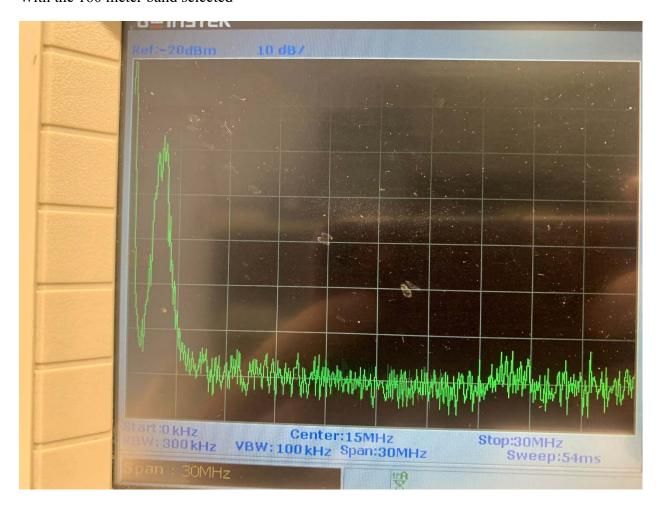
No attenuation on the 160 meter band, remaining spectrum attenuated > 50db
