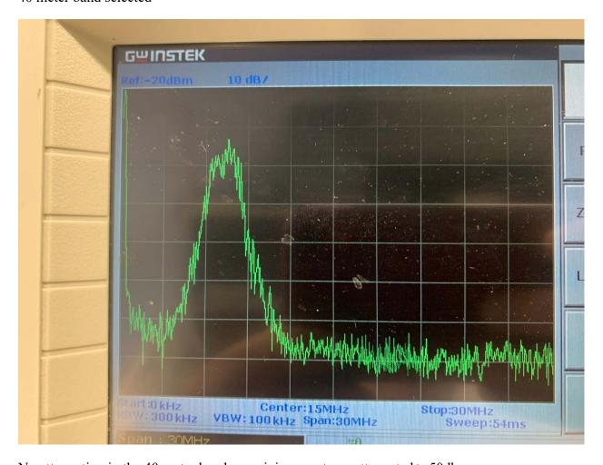
No attenuation in the 40 meter band, remaining spectrum attenuated > 50db
