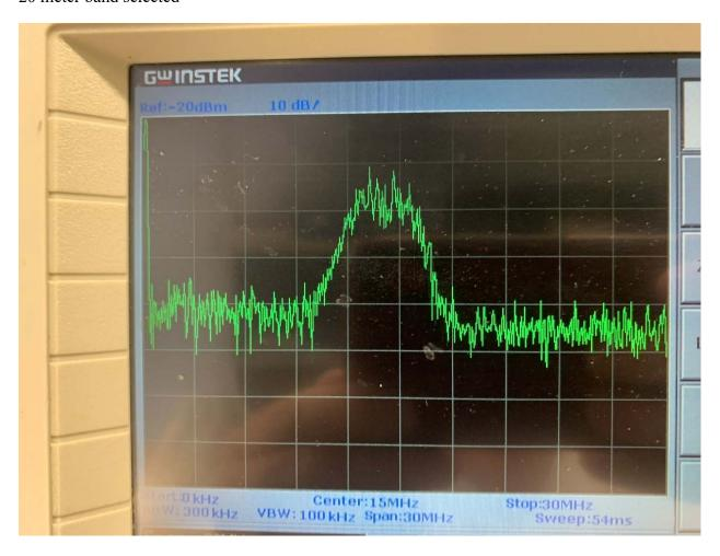
No attenuation in the 20 meter band, remaining spectrum attenuated > 30db
