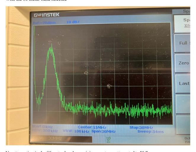
No attenuation in the 80 meter band, remaining spectrum attenuated > 50db
