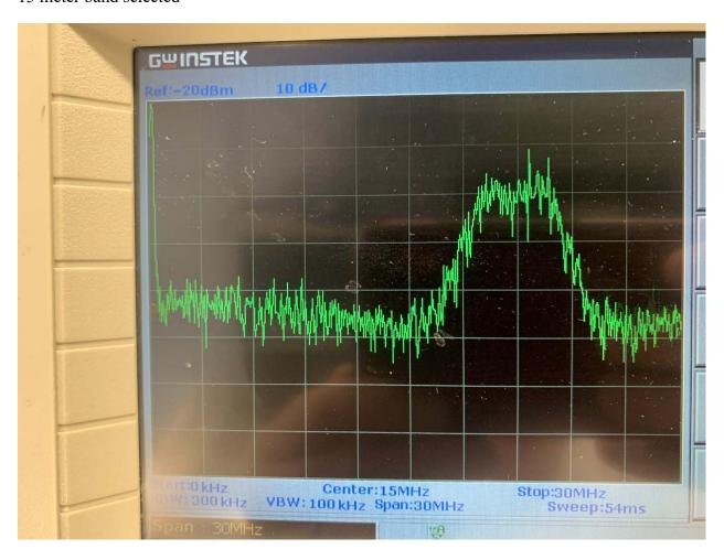
No attenuation in the 15 meter band, remaining spectrum attenuated > 30db
