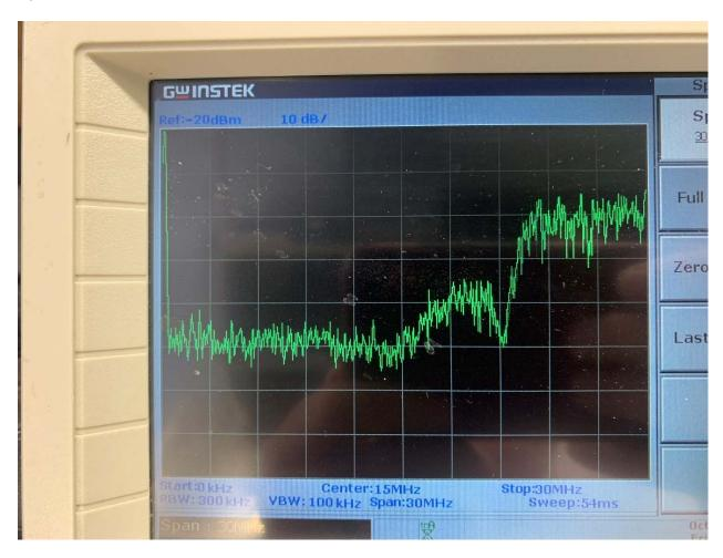
No attenuation in the 10 meter on up band, 15 meter band attenuation > 20db, 20 meter and lower band attenuation > 30db
